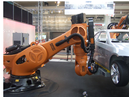
KUKA KR 1000 titan (charge max: 1300 kg)
