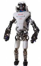
TEAM WPI-CMU Robot: WARNER (Atlas) Country: USA DOB: 2013 Height: 190 cm Weight: 180 kg
