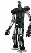
TEAM ROBOTIS Robot: THORMANG Country: South Korea DOB: 2013 Height: 160 cm Weight: 60 kg
