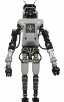
TEAM TRAC LABS Robot: Hercules (Atlas) Country: USA DOB: 2013 Height: 190 cm Weight: 180 kg
