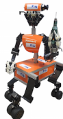
TEAM NIMBRO RESCUE Robot: Momaro Country: Germany DOB: 2015 Height: 150 cm Weight: 60 kg
