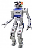
TEAM KAIST Robot: DRC-HUBO Country: South Korea DOB: 2014 Height: 180 cm Weight: 80 kg
