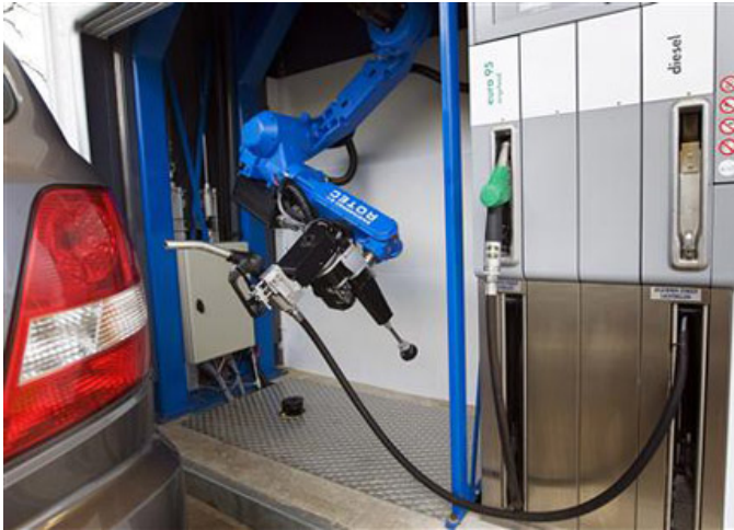
Robot pompiste ("pitstop") https://rotec-engineering.nl
