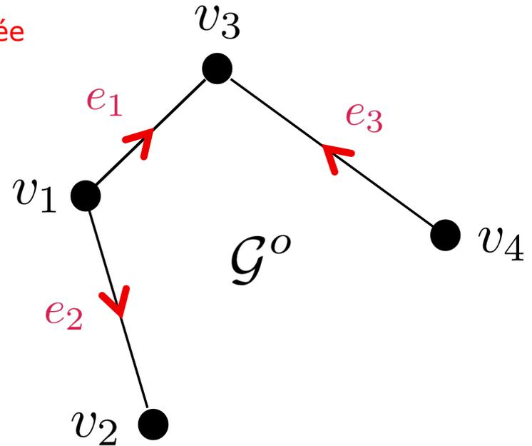
$$\mathbf{D}(\mathcal{G}^o) = \begin{bmatrix} e_1 & e_2 & e_3 \\ -1 & -1 & 0 \\ 0 & 1 & 0 \\ 1 & 0 & 1 \\ 0 & 0 & -1 \end{bmatrix} \begin{matrix} v_1 \\ v_2 \\ v_3 \\ v_4 \end{matrix}$$
