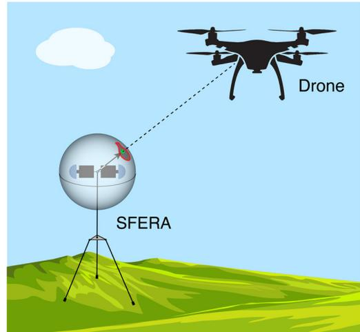
Fig. 1. *Conceptual illustration of SFERA.* The sensor is used here for event-based omnidirectional detection and tracking of a flying object (e.g. a drone).
