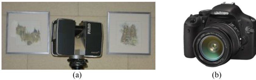
Figure 2: Tools used for the digitization of the cathedral of Amiens in France. (a) Laser scanners measure the structure with high precision. (b) Cameras acquire image that can also be used for computing structure from multiple images in addition to the color measurement.
