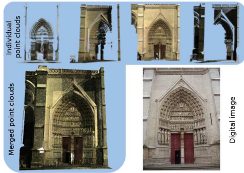
Figure 2: Color problems resulting of the point clouds merging and the scanner camera low quality
